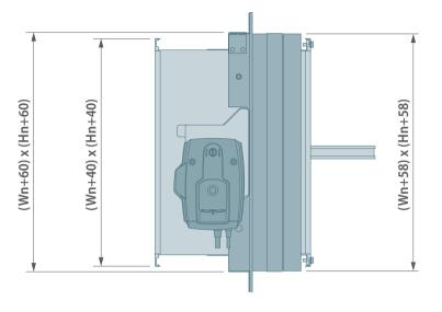
Universal screw Ø6 x 50mm to be fitted into the provided screw openings in the flange (max. 7pc. for the largest damper size).
